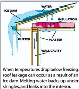
When temperatures drop below freezing, roof leakage can occur as a result of an ice dam. Melting water backs up under shingles, and leaks into the interior.
